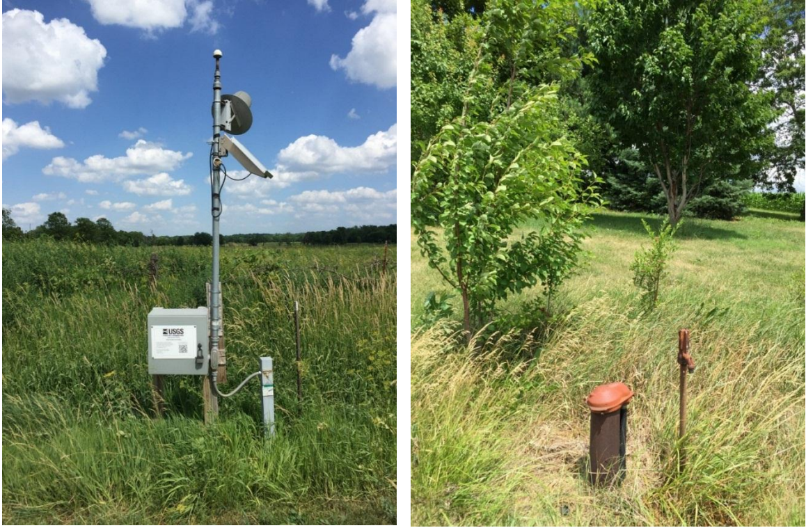
Figure 9 Photographs of examples of an agriculture monitoring well (left) and a domestic well (right) sampled for this project. The agriculture monitoring well shown is also equipped with groundwater level monitoring equipment. Photos by Kymm Barnes, Hydrologist, U.S. Geological Survey.
