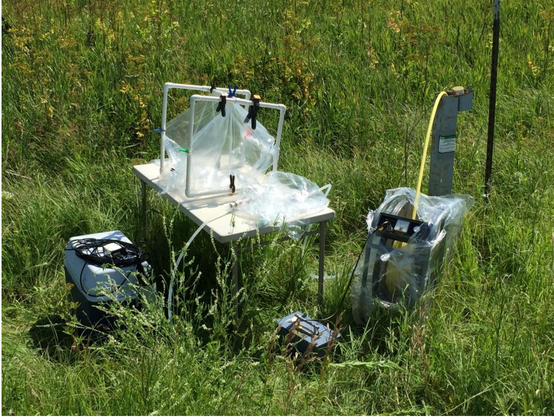
Figure 10 Example of a USGS agriculture monitoring well water quality sampling setup using a submersible gear pump. Photo by Kymm Barnes, Hydrologist, U.S. Geological Survey.
