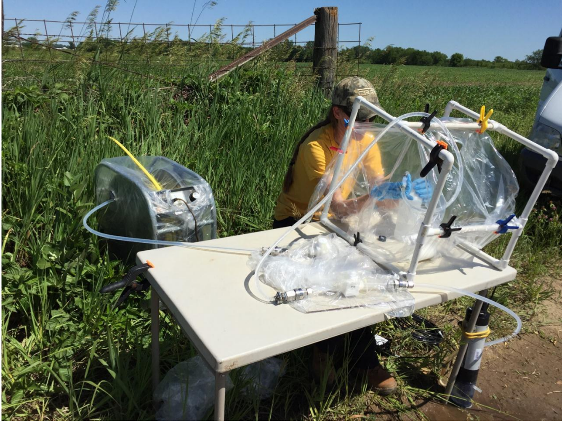
Figure 11 A photo of me collecting water quality samples from an agriculture monitoring well, following USGS sampling protocol. Photo by Kymm Barnes, Hydrologist, U.S. Geological Survey.
